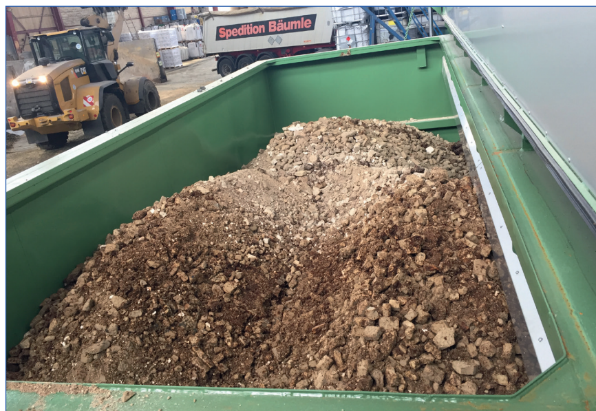
Fig. 3 – Extremely dry air combined with appropriate air routing ensures uniform drying of the sludge. Drying can reduce sludge weight and volume by as much as 60 percent.
